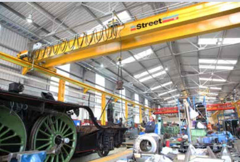
ZX double girder cranes helping to refurbish heritage steam locomotives.
